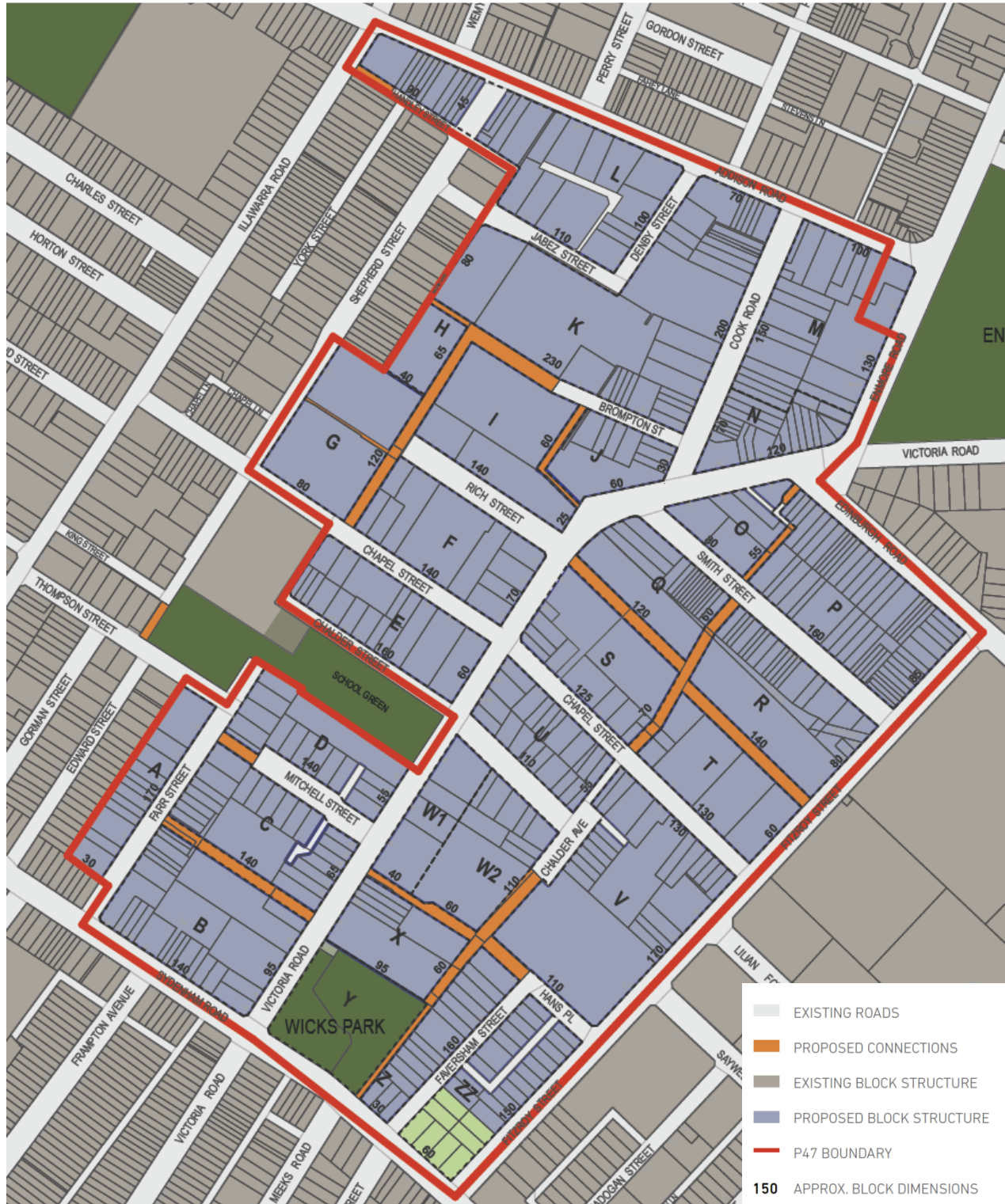
Figure 16 – Proposed new road connections and block structures
